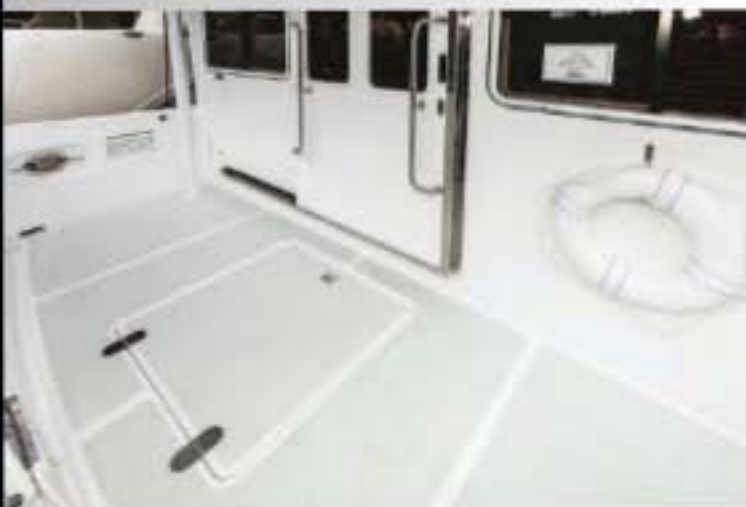
COVERED, NON-SKID COCKPIT WITH HIGH, SECURE BULWARKS.
