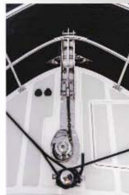
ABOVE: STAINLESS SAFETY RAILS ON FOREDECK, AND NO EXTERIOR TEAK. LEFT: STAINLESS BOW PULPIT, WINDLASS, AND SAMSON POST DRESS UP THE BOW.
