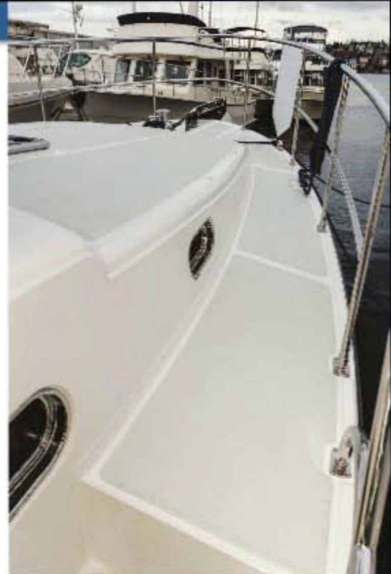
ABOVE: STAINLESS SAFETY RAILS ON FOREDECK, AND NO EXTERIOR TEAK. LEFT: STAINLESS BOW PULPIT, WINDLASS, AND SAMSON POST DRESS UP THE BOW.
