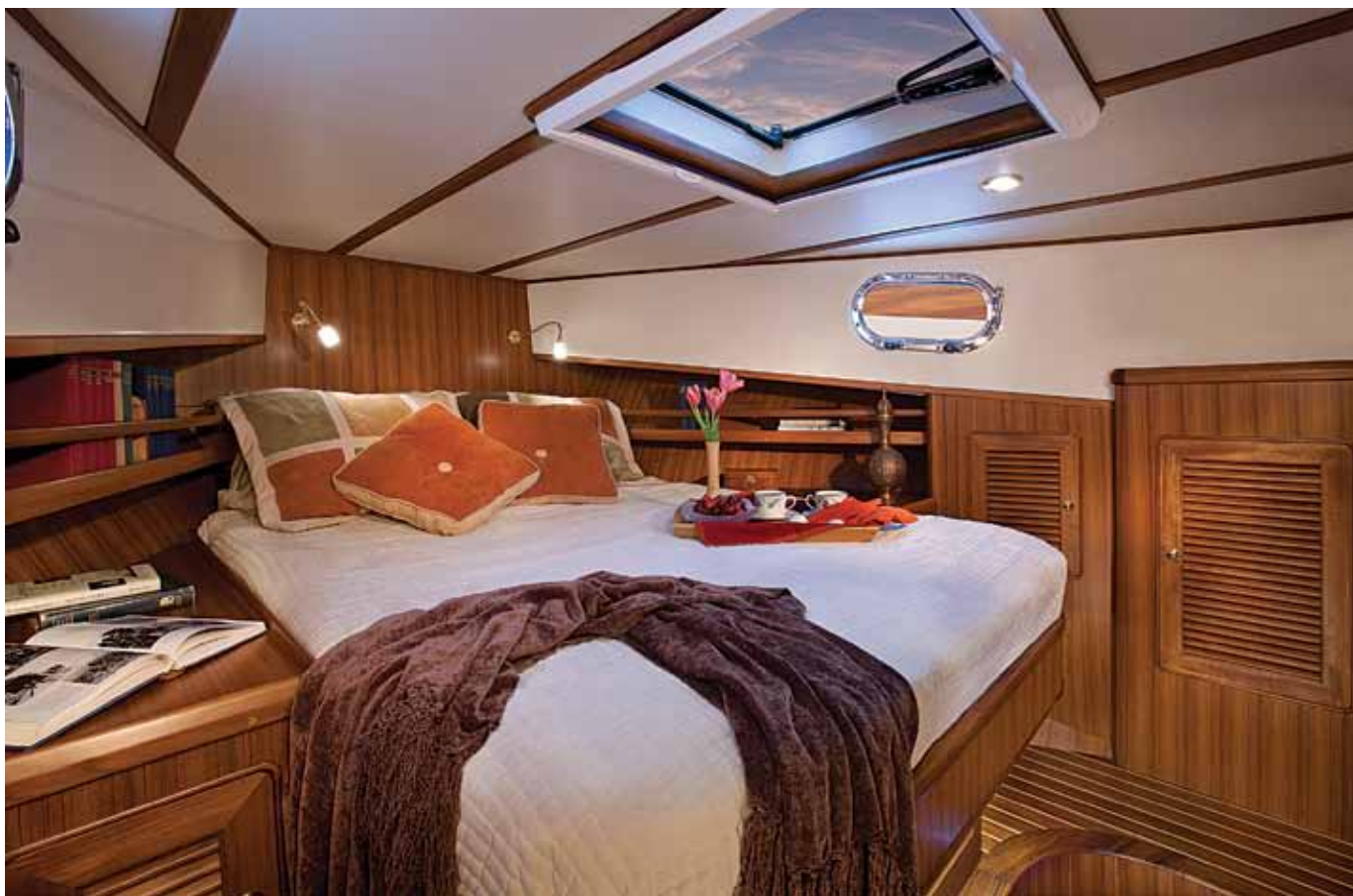
An overhead skylight hatch and two opening portlights help illuminate and freshen the forward master stateroom. Note the louvered cabinet doors for ventilating lockers, as well as the handy bookshelves with sea rails.
